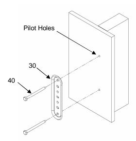
Figure 1. Secure Wall Bracket
